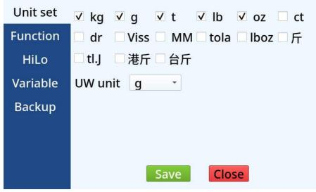
The column on the left is setting classification. It includes unit setting, function setting, Hi-Lo setting, variable edit, backup restore.
